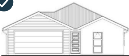
Acceptable double gable roof
